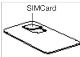
Remove it from its surround by carefully pushing it out. The SIM Card's contacts are easily damaged, take care when handling it and try to avoid touching the golden contacts.
